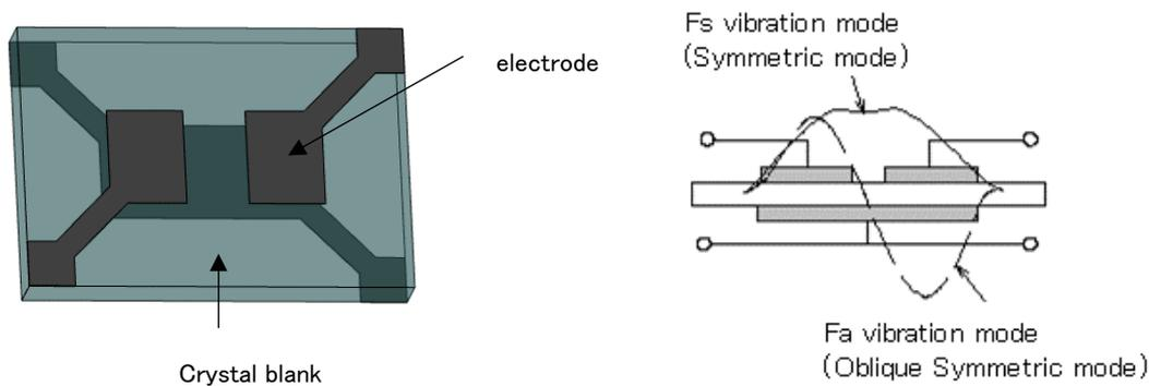
Fig.2: MCF configuration and Vibration mode outline
