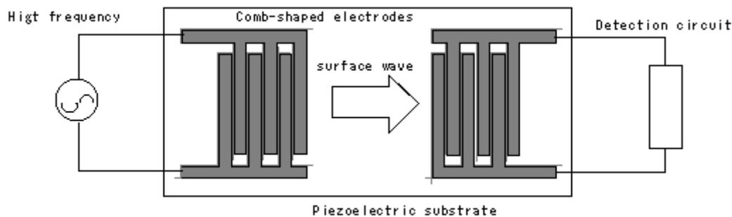
Fig.1: SAW Filter configuration
